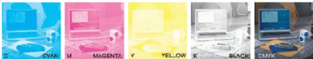
A color image is separated into CMYK. When printed on paper, the original image is recreated.
